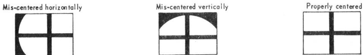
Fig. 17. Effects of centering on vidicon scanning.
