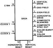
V<sub>SS</sub> = Pin 16 V<sub>DD</sub> = Pin 9 V<sub>GG</sub> = Pin 8
